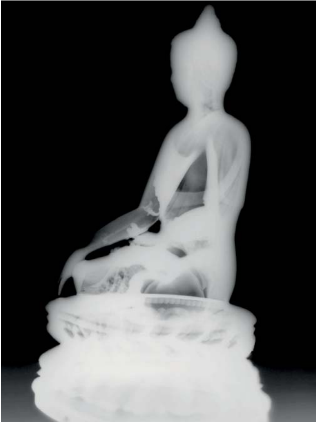
Figure 5. X-radiograph of the Buddha from the side
